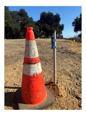
**Ground Temperature Data collection – full sun:** Through the entire period of the heatwave the thermocouple was located in a sealed 1" PVC tube 4ft long. The PVC was buried vertically with the thermocouple probe 3ft below the surface. The soil was bare at the surface and compacted sandy loam soil with no ground cover.
